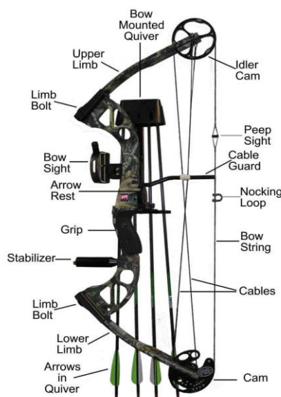
Figure 8- Parts of a compound bow.
